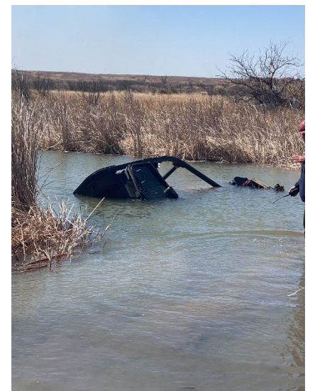
The dozer submerged in the water after the “rip-rap” gave way.
